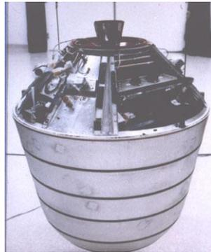
**Fig. 3: Corona Style Reentry Vehicle**
