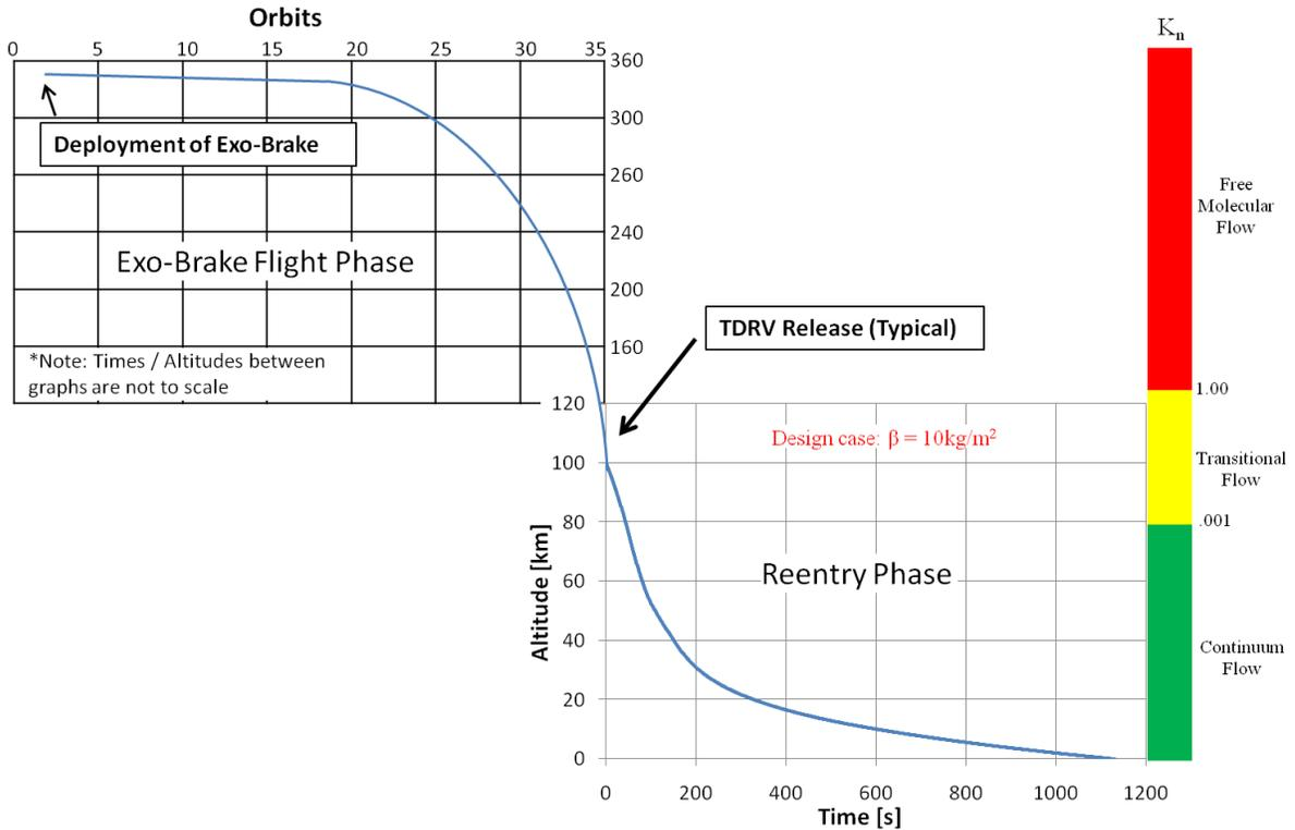
Fig. 7: Sample SPQR Altitude vs. Orbit/Time Plot
