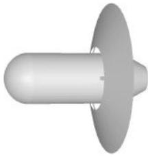
Figure 3. The basic SCRAMP probe geometry.
