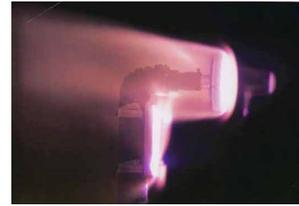
Figure 12. Arc-jet test of shock interaction and translation stage at Mars entry conditions.
