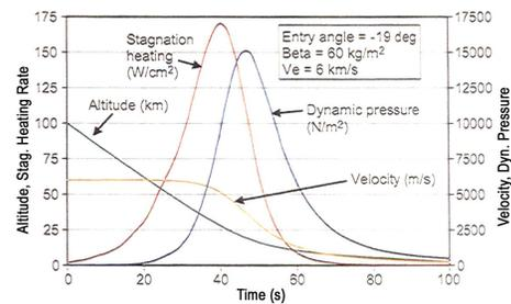
Figure 13. Entry heating calculations for Mars entry case.
