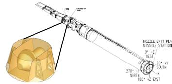
Figure 11. SOAREX VI Payload Ejection System.
