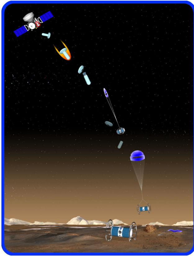
Figure 1. Atromos mission sequence (S/C separation, entry, descent and landing).
